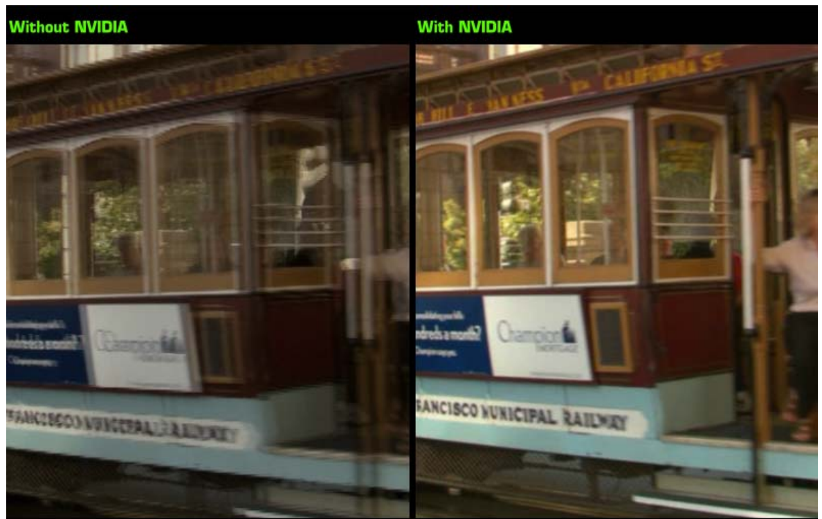
Figure 11. The 3:2 Pull-Down Correction Recovers Original Content and Displays Clean Images Frame After Frame
