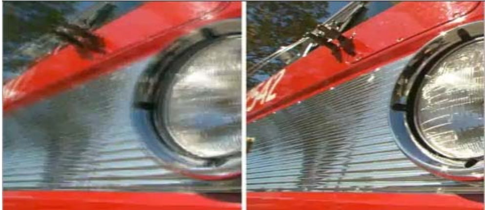
Figure 12. Artifacts in Video Image (Left) vs. No Artifacts with PureVideo Edit Detection and Correction (Right)
